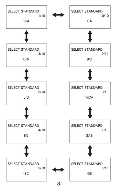
After selecting standard, press to confirm then press to set BATTERY RATING.
